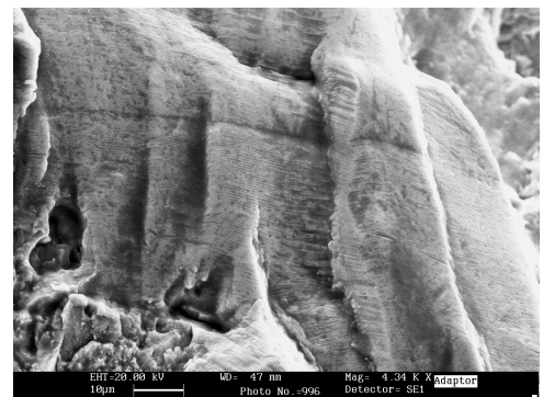
Fig.7: High magnification SEM images showing presence of fatigue striations on the fracture surface of the adapter
